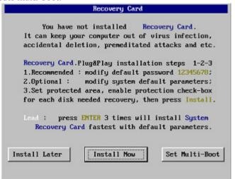
5.4 Preset Multi-Boot is an independent pretreatment module and can carry out multi-system booting on single hard disk. If you want to partition one hard disk into many completely independent bootable disks, you
