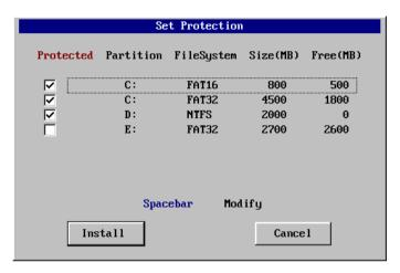
5.9 After completing setting of protection area, you can press Enter key or select "Install" button. Recovery Card shall analyze hard disk and save system parameters, and restart the computer after a while. If automatic recovery of CMOS data is enabled, Recovery Card will ask to shut off computer for a moment and restart it automatically three times. Now the installation of Recovery Card is completely finished.
